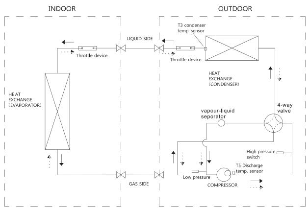
**NOTE:** In heating mode, the throttling device is outdoor unit piston. In cooling mode, the throttling device is indoor unit TXV or piston.
